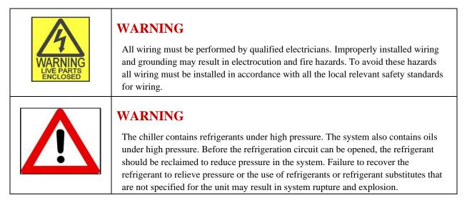
Refrigerants have a narcotic effect when inhaled in high quantities. Should a leak occur of the refrigerants then the room should be vacated and should only be re-entered after suitable ventilation.
